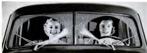
Turning a dashboard switch sends a stream of water across the windshield
